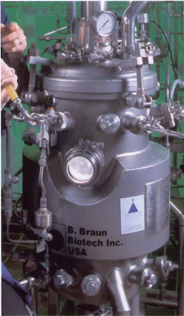
▲ This is a bioreactor and is used to grow bacteria which have recombinant DNA.
